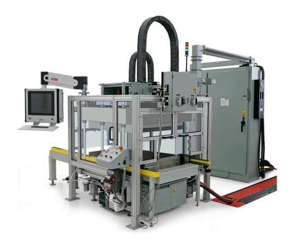
185 Ton RTM & SQRTM press with heating and cooling capability.
