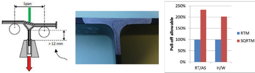
Figure 21. Pull-off test on cocured spar-skin junction.
