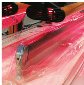
Hot-forming of nose and spars
