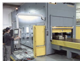
SQRTM curing in press
