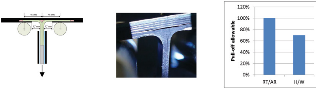
Figure 4. Pull-off tests on rib foot - skin connection.
