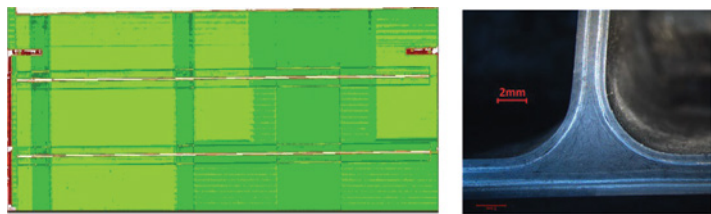
Figure 13. C-scan and micrography from the lower skin demonstrator with cocured spars.
