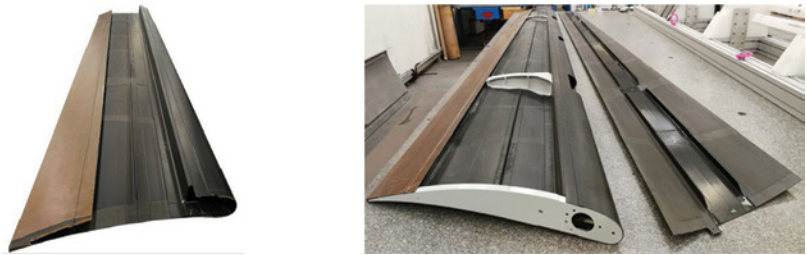
Figure 17. Flap lower skin demonstrator with cocured spars, nose and trailing edge (4,3 m).
